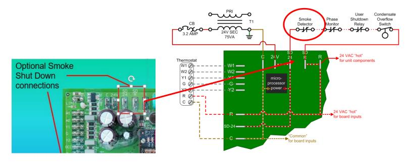
Anything wired between SD 24 and SD R that opens will shut unit off but leaves board display powered so alarm "shut down due to smoke detector" will be displayed.
