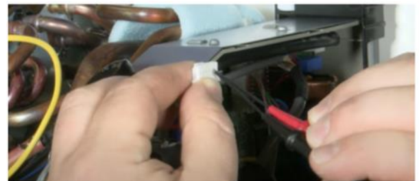
Test with needlepoint leads on the 2 silver tabs
