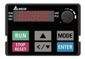
Normal display (home screen) on the Delta VFD can be rotated between the displays listed below, by using the **MODE** button.
