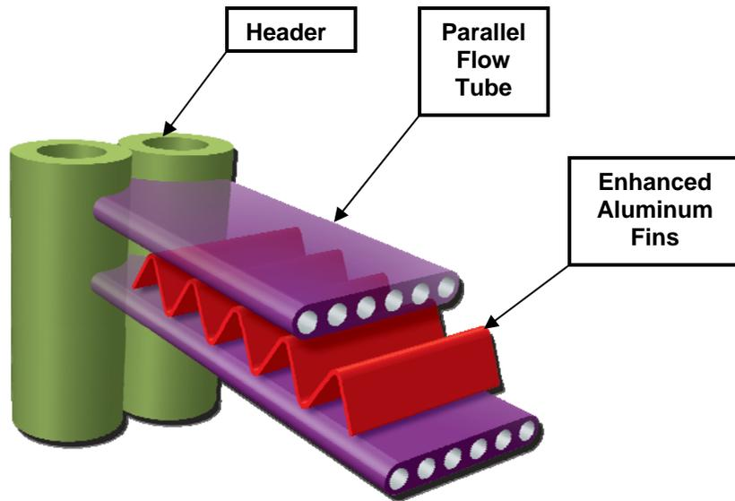
FIGURE 3 – Basic Microchannel Coil Construction
