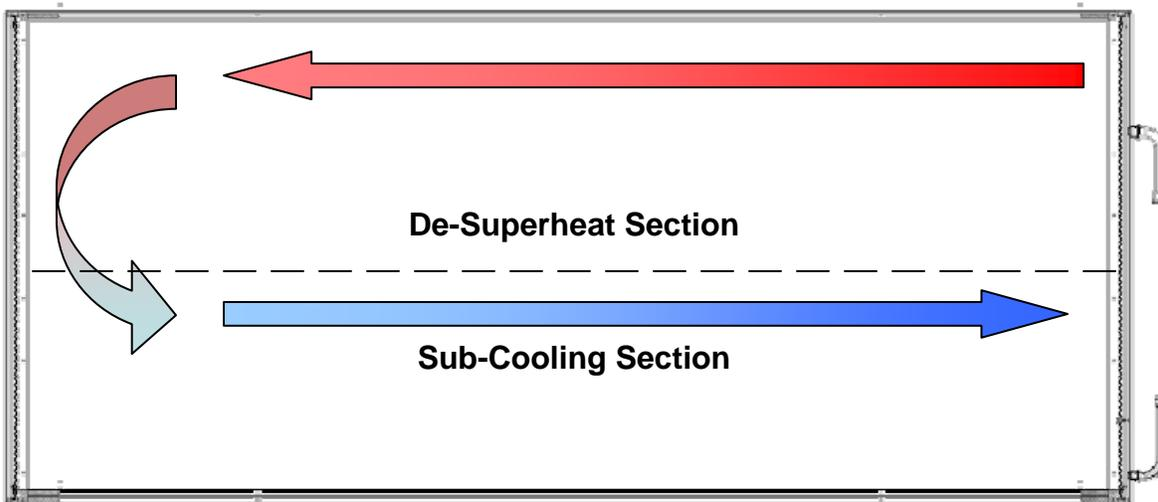
FIGURE 4 – Typical Microchannel Refrigerant Flow
