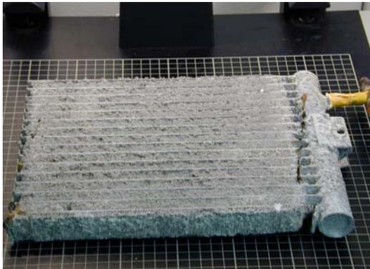
FIGURE 5 – Microchannel coil at 7000 hrs
