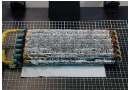
FIGURE 6 – TF coil at 1000 hrs
