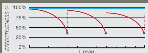
Compare this to the efficiency of standard electronic air cleaners which drop off repeatedly throughout the year, never regaining their original efficiency, even after filter replacement or cleaning.
